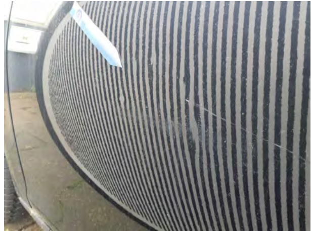
Beschädigung 10: Tür vorn links: Tür - Delle / Lackschaden - Smart Repair
